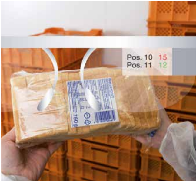
The latest option: Pick-by-Vision, in which the pickers wear data glasses where all the information for distribution is visible in the inner surface
