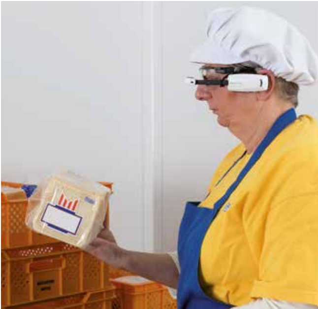
Pick-by-Vision using data glasses is recommended for error-free order-picking of easily damaged snacks even in confined spaces
