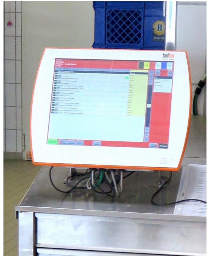
The "command post" where the order pickers call up customers for whom they are now collecting goods
